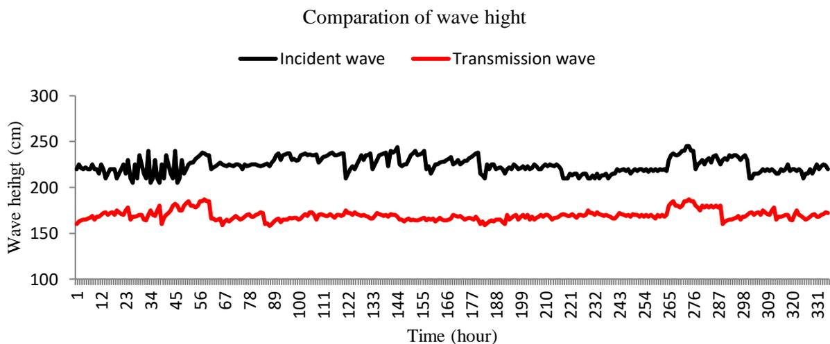
Figure 3. Comparison of Incident Wave Height ( $H_i$ ) and Transmission Wave Height ( $H_t$ )
